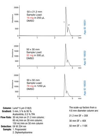
The maximum load for each column must be adjusted based on the column diameter but each column provides the same purification capability and performance.
