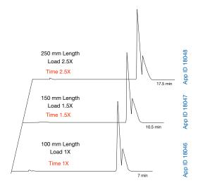
Increasing the column length and increasing the sample load proportional to the length reduces the number of runs or cycles and generates fewer fractions to evaluate. The longer column is also more forgiving with the injection volume. The throughput remains constant (grams/hour).
