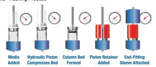
Axial compression technology is incorporated into manufacturing pre-packed short prep columns. Once the column is formed, the column hardware is fully assembled leaving the piston in place and the media fully compressed before the pneumatic ram is removed.
