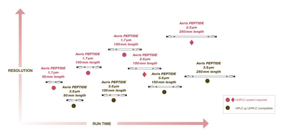
The family of Aeris PEPTIDE XB-C18 columns is designed to provide versatility for the development of peptide separation methods. Depending on your resolution, throughput goals, and pressure capabilities of your system, you can choose from three particle sizes with unique performance attributes, as well as several column lengths to select the most suitable column for seamless method development and excellent results.
