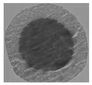
Cross section of an Aeris core-shell particle
